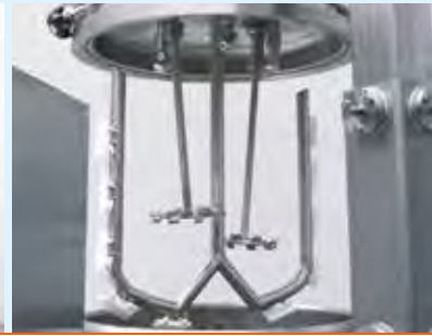
domed agitator with dissolver
